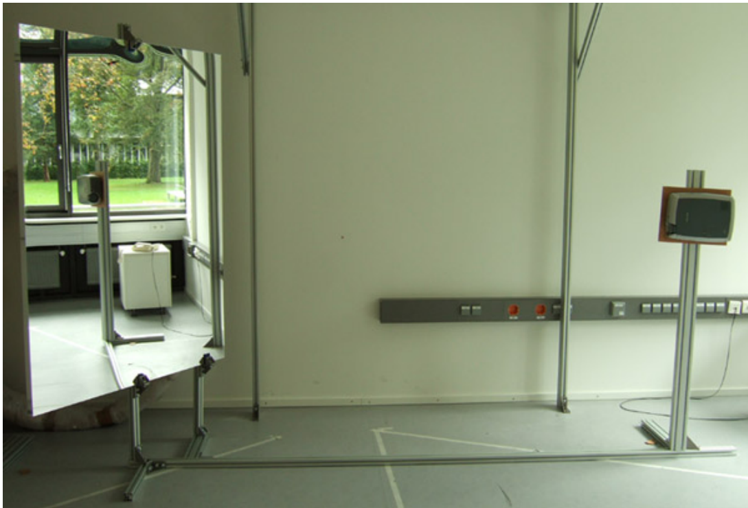
Fig. 6) Projector/mirror connection for the cylinder projection. You can see the mounting rack for the aluminum mirror and the projector turned around the longitudinal axis. In order to fix the projection distance, a further bar from the aluminum profile is used.
